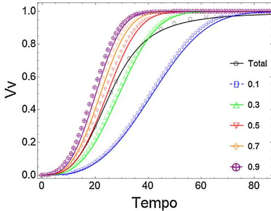
**Fig. 1 – Transformation kinetics for inhomogeneous nucleation and homogeneous growth velocity.** The transformation kinetics, the mean volume density against time, is slower at the bottom that has a smaller nuclei density than at the top that has a high nuclei density. The solid lines represent the analytical results. The dots represent the simulated data.
