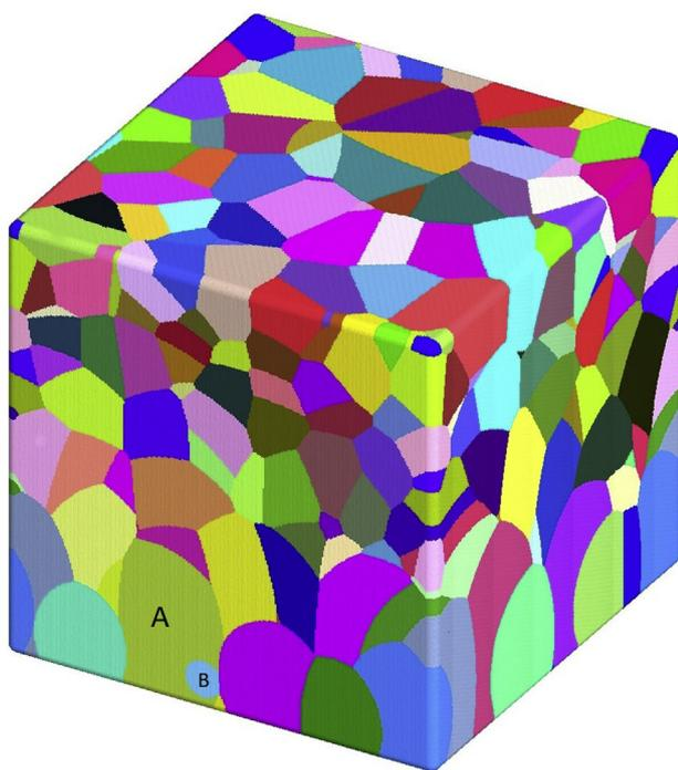
**Fig. 4 – 3D representation showing the simulated microstructure with homogeneous nucleation and inhomogeneous growth velocity. The growth velocity was higher at the top of the specimen. As a result, the final grain size is smaller at the top than at the bottom.**
