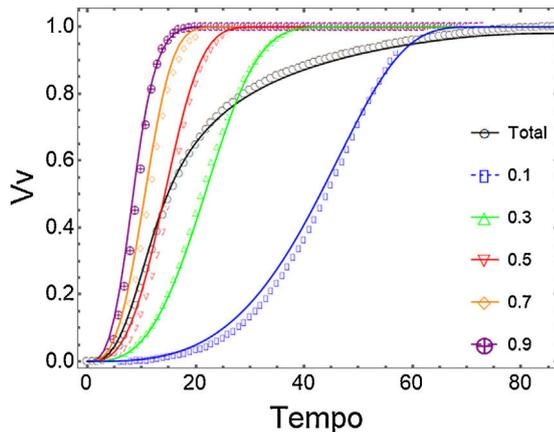
**Fig. 2 – Transformation kinetics for homogeneous nucleation and inhomogeneous growth velocity.** The transformation kinetics, the mean volume density against time, is slower at the bottom that has a smaller growth velocity than at the top that has a high growth velocity. The solid lines represent the analytical results. The dots represent the simulated data.
