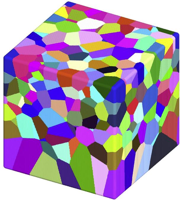
**Fig. 3 – 3D representation showing the simulated microstructure with inhomogeneous nucleation and homogeneous growth velocity.** The nuclei density was higher at the top of the specimen. As a result, the final grain size is smaller at the top than at the bottom.
