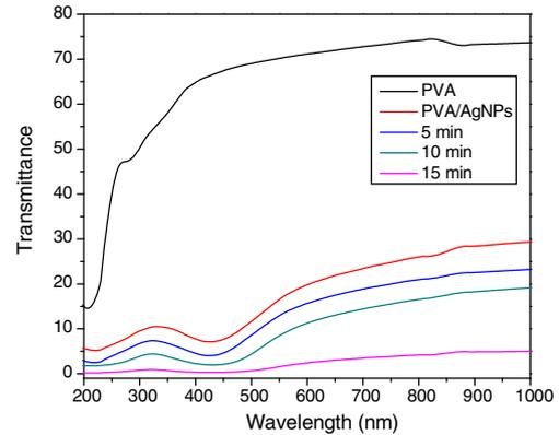
**Fig. 8 – UV-visible transmittance spectra for pure PVA and PVA/Ag nanocomposite films before and after irradiated to different times of nanosecond laser (5, 10, and 15 min).**
