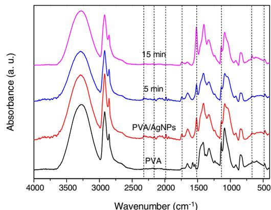
**Fig. 2 – FT-IR absorption spectra for pure PVA and PVA/Ag nanocomposite films before and after irradiated to different times of nanosecond laser (5, 10, and 15 min).**
