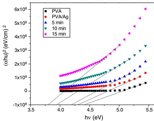
**Fig. 7 – Plots of  $(\alpha h\nu)^2$  versus photon energy ( $h\nu$ ) for pure PVA and PVA/Ag nanocomposite films before and after irradiated to different times of nanosecond laser (5, 10, 15 min).**
