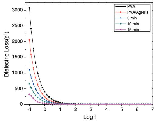
**Fig. 10 – Typical plots of variation of imaginary part of the dielectric constant ( $\epsilon''$ ) with frequency for pure PVA and PVA/Ag nanocomposite films before and after irradiated to different times of nanosecond laser (5, 10, 15 min) at room temperature.**
