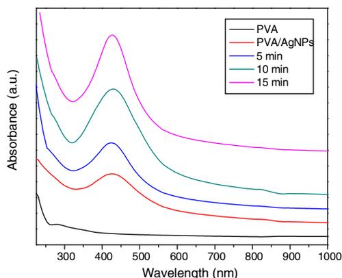
**Fig. 3 – UV-visible absorbance spectra for pure PVA and PVA/Ag nanocomposite films before and after irradiated to different times of nanosecond laser (5, 10, and 15 min).**
