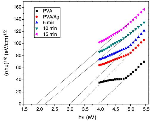
**Fig. 6 – Plots of  $(\alpha h\nu)^{1/2}$  versus photon energy ( $h\nu$ ) for pure PVA and PVA/Ag nanocomposite films before and after irradiated to different times of nanosecond laser (5, 10, 15 min).**
