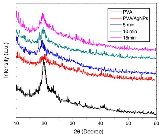
**Fig. 1 – XRD patterns for pure PVA and PVA/Ag nanocomposite films before and after irradiated to different times of nanosecond laser (5, 10, 15 min).**
