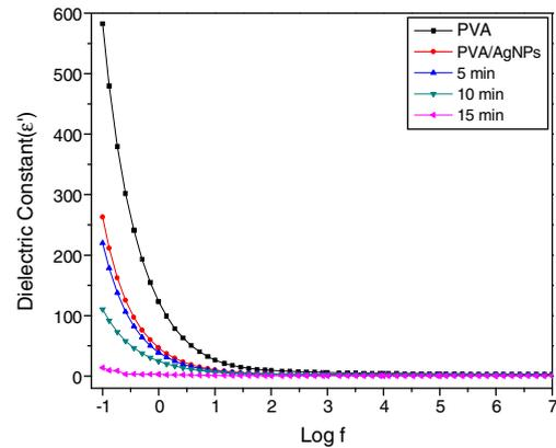
**Fig. 9 – Typical plots of variation of real part of the dielectric constant ( $\epsilon'$ ) with frequency for pure PVA and PVA/Ag nanocomposite films before and after irradiated to different times of nanosecond laser (5, 10, 15 min) at room temperature.**
