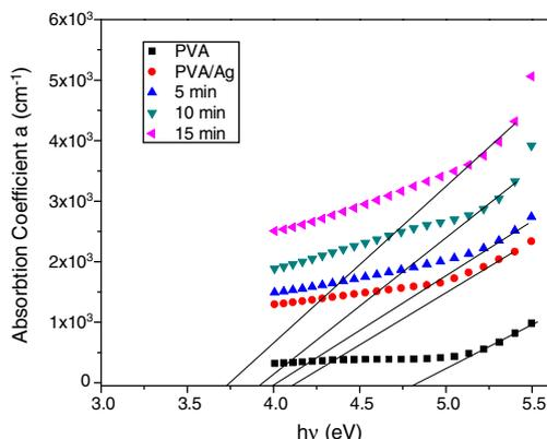
**Fig. 5 – Relation between absorption coefficient ( $\alpha$ ) versus ( $h\nu$ ) for pure PVA and PVA/Ag nanocomposite films before and after irradiated to different times of nanosecond laser (5, 10, and 15 min).**
