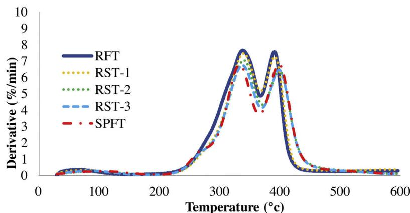
Fig. 5 – DTG of RF/SPF hybrid composites.
