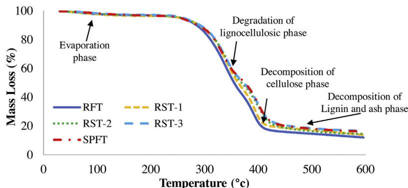
Fig. 4 – TGA of RF/SPF hybrid composites.
