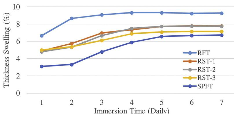
Fig. 3 – Thickness swelling of RF/SPF hybrid composites.
