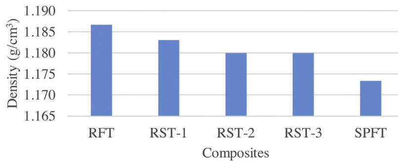
**Fig. 1 – Density of RF/SPF hybrid composites.**
