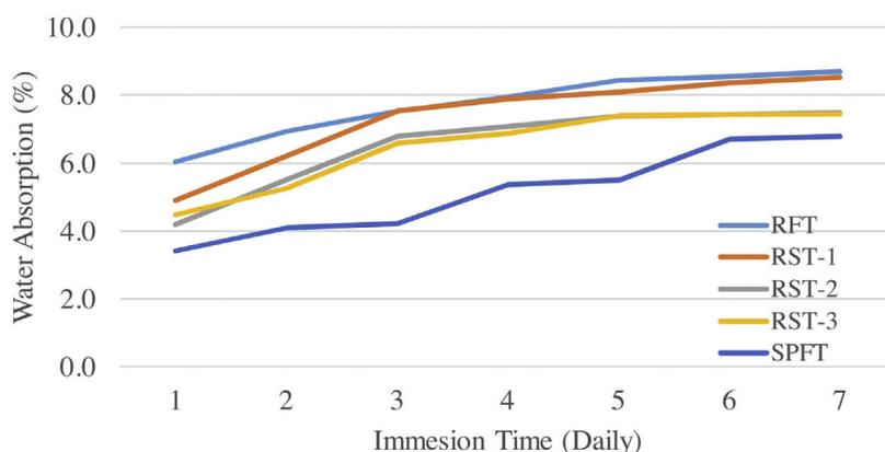
Fig. 2 – Water absorption of RF/SPF hybrid composites.
