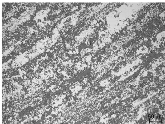
**Figure 4 – Microstructure of the ferritoscope calibration sample. The calibration pattern define the ferrite content in the sample as 30.40%, which diverge from 51.4% of ferrite achieved by metallographic quantification with optical microscopy.**
