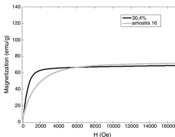
**Figure 5 – Magnetization curves. In gray, the curve of the sample 16, as-annealed, and in black the magnetization curve of the calibration sample with 30.40% of ferrite used for the ferritoscope calibration.**
