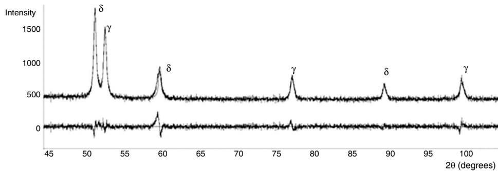
Figure 1 – XRD spectrum of sample 16 with 49.7% of ferrite.
