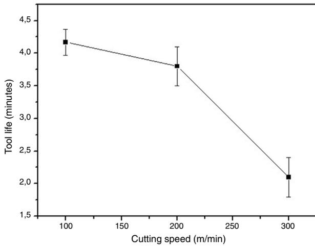
**Fig. 2 – Cutting speed vs. tool life of the 70% AlN sintered at 1800 °C.**
