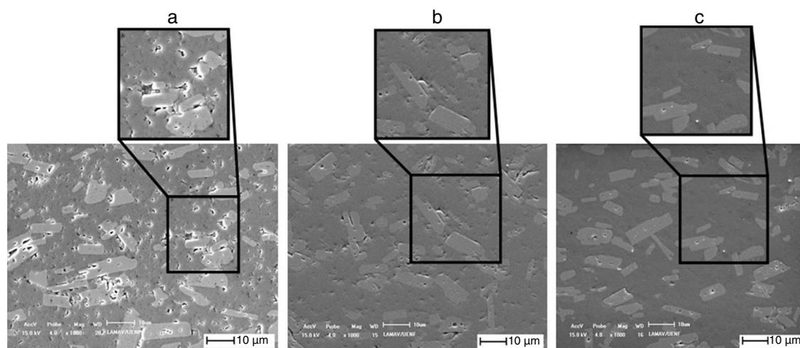
**Fig. 1 – SEM micrograph of 70 wt% of AlN samples sintered in different temperatures: (a)  $1600\ ^\circ C$ ; (b)  $1700\ ^\circ C$ ; and (c)  $1800\ ^\circ C$ .**
