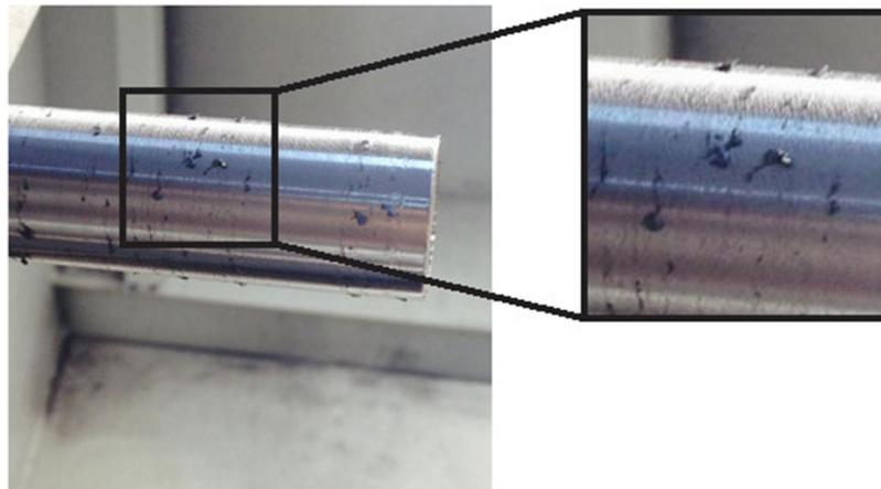
**Fig. 3 – Machined surface using 70 wt% TiB<sub>2</sub> composite as cutting tool.**
