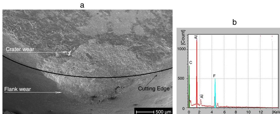
**Fig. 4 – SEM (a) and EDS (b) of a 70 wt% AlN wear crater ( $V_c = 300$  m/min).**
