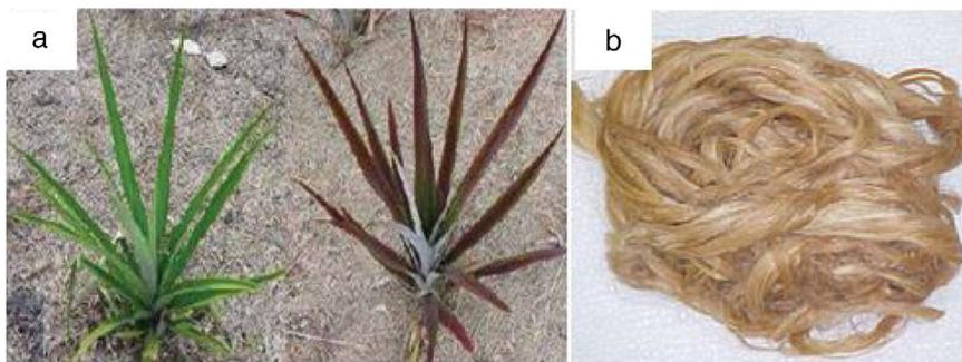
Fig. 1 – (a) Curaua plant and (b) curaua fiber processed and ready for use.
