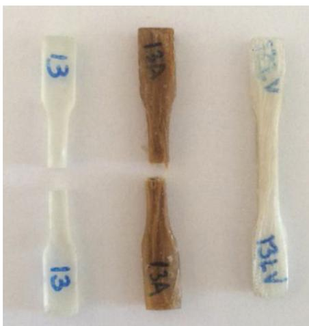
**Fig. 4 – Typical tensile ruptured specimens with 0% of fiber, 30% curaua fiber and 30% glass fiber reinforced epoxy composites.**
