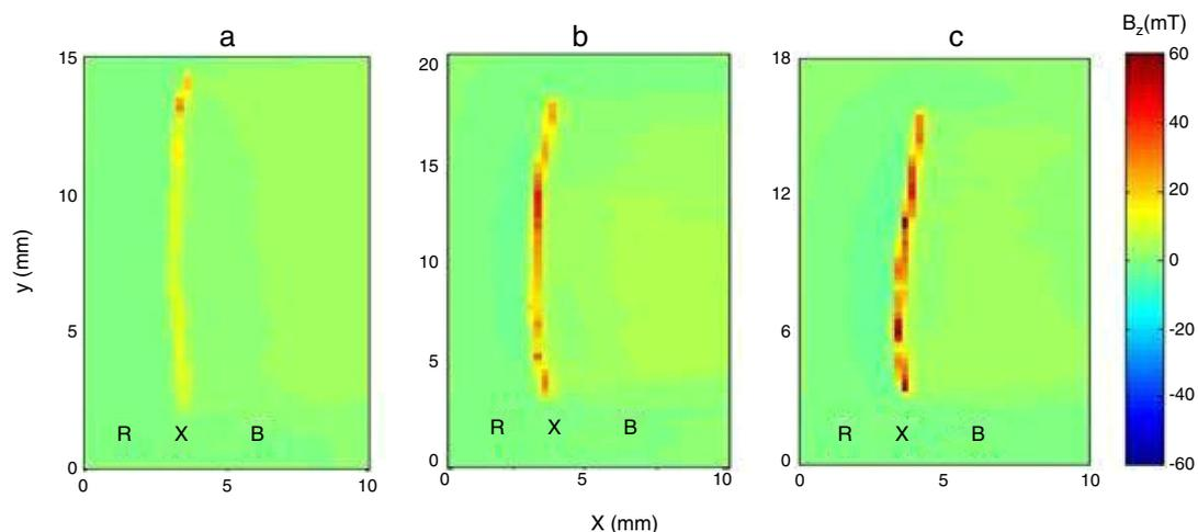
**Fig. 7 – Magnetic response of external surface of the three samples under a 400 mT field, applied perpendicularly to the sample surface. Sample with: (a) aging state II – A1, (b) aging state IV – A2 and (c) aging state V – A3. The region (B) represents the bulk of sample, (X) the external surface and (R) the resin in which the samples were embedded.**
