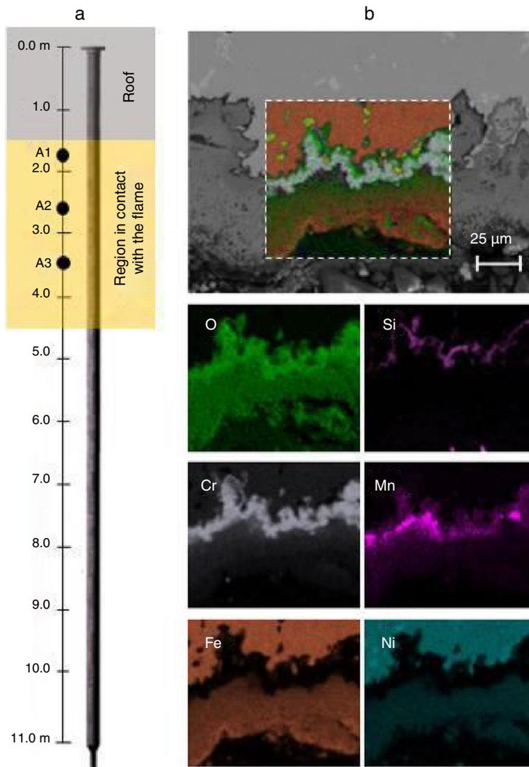
Fig. 2 – (a) Tube scheme showing the position of samples A1, A2 and A3 removed from the reformer column. (b) EDS mapping of sample A2, showing the typical chemical elements present on the oxide scale and their distribution, overlaid at the backscattering image.
