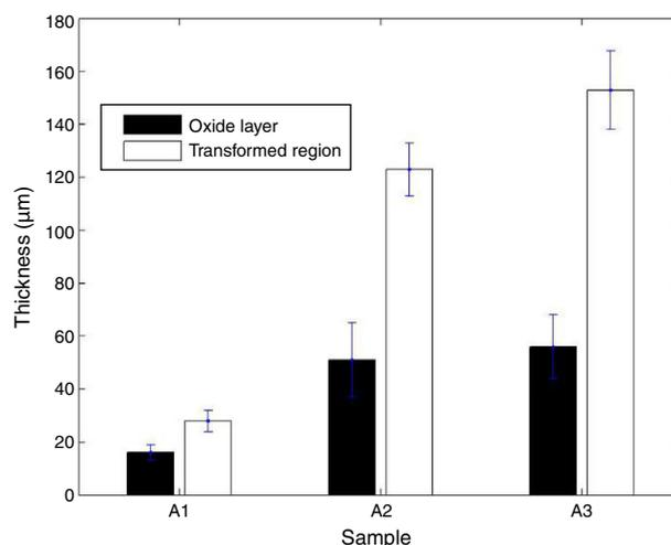
**Fig. 5 – Average thickness of oxide layer and transformed region (in µm) for samples A1, A2 and A3.**
