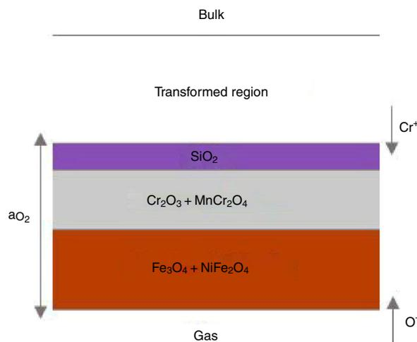
**Fig. 4 – Phases distribution model for the external oxide scale formed at modified HP steel tubes used in steam reforming furnaces.**
