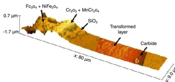
**Fig. 6 – Scan line topography, showing the phases presents on it and the ferromagnetic response of the transformed region and the paramagnetic response of the carbide.**
