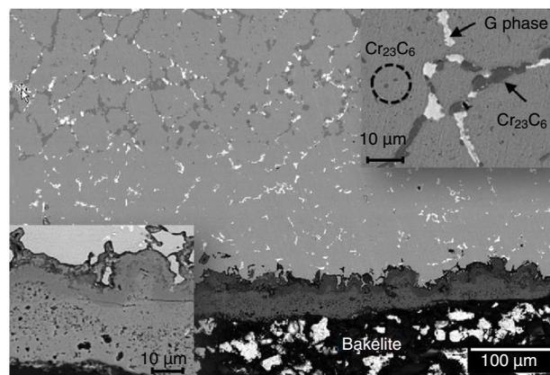
**Fig. 1 – Backscattered electron mode image of sample A3, showing the typical morphology of the HP tube external surface.**
