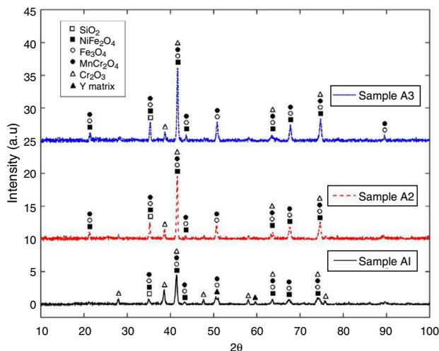
**Fig. 3 – X-ray diffraction results, showing the oxides presents in the external oxide scale of the samples A1, A2 and A3.**
