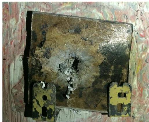
**Fig. 4 – Typical aspect after ballistic test of MAS targets with second layer of 30 vol% jute non-woven mat reinforced polyester composite.**
