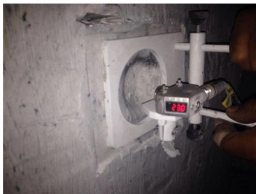
**Fig. 3 – Depth of indentation in the clay witness measured with laser sensor caliper.**
