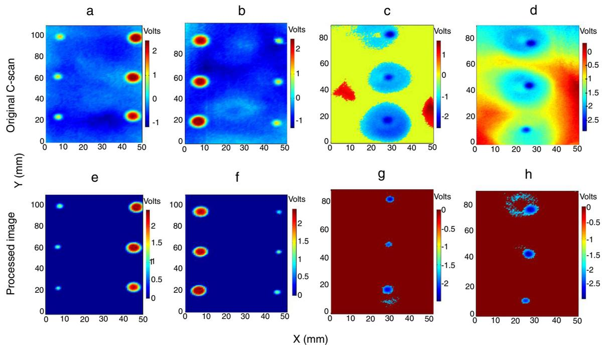
**Fig. 1 – Original C-scan map: (a) sample A coated with EP  $972 \pm 55 \mu\text{m}$ ; (b) sample B coated with EA  $376 \pm 60 \mu\text{m}$ ; (c) sample C coated with EP  $582 \pm 125 \mu\text{m}$ ; (d) sample D coated with EP  $670 \pm 140 \mu\text{m}$ . Processed image of samples: (e) A; (f) B; (g) C; (h) D.**
