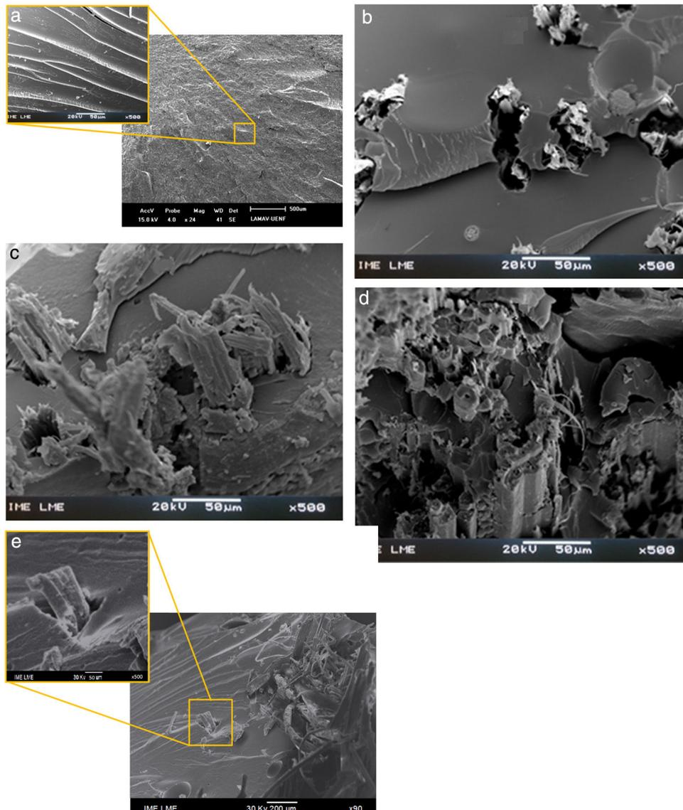
**Fig. 7 – SEM tensile fractograph of (a) plain polyester, (b) 10, (c) 20, (d) 30 and (e) 40 vol% mallow fabric polyester matrix composite.**
