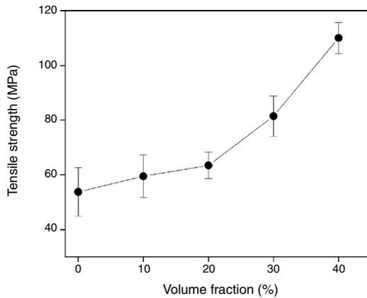
**Fig. 4 – Variation of tensile strength of polyester composites as a function of volume fraction of mallow fabric.**
