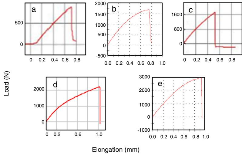
**Fig. 3 – Typical load vs. elongation curves of tensile specimens with (a) zero (0%), (b) 10, (c) 20, (d) 30 and (e) 40 vol% of mallow fabric.**
