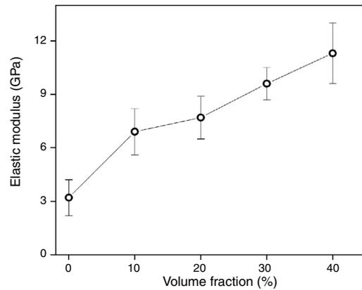
**Fig. 5 – Variation of elastic modulus of polyester composites as a function of the volume fraction of mallow fabric.**
