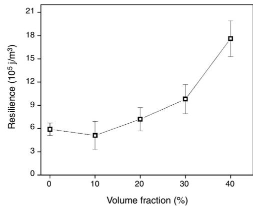
**Fig. 6 – Variation of the polyester composite resilience with the volume fraction of mallow fabric.**
