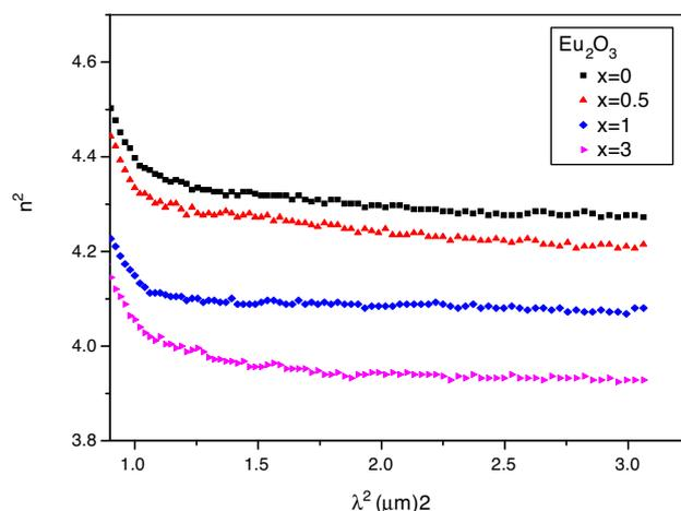
**Fig. 8 – The relation between ( $n^2$ ) and ( $\lambda$ )<sup>2</sup> as function of  $\text{Eu}_2\text{O}_3$ .**
