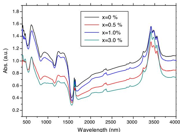
**Fig. 2 – FTIR for base glass and glass doped with x mol% Eu<sub>2</sub>O<sub>3</sub>.**
