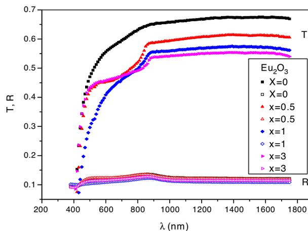
**Fig. 3 – The transmittance T(λ) and the reflectance R(λ) spectra for ZnO boro-tellurite glasses doped with x Eu<sub>2</sub>O<sub>3</sub>.**
