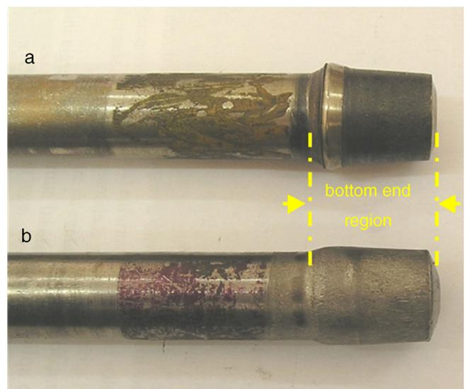
**Fig. 5 – The bottom end region of (a) an unused (wear-free) and (b) a wearing rod part.**
