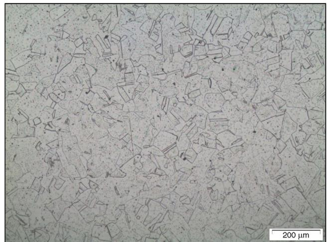
**Fig. 3 – Optical micrograph of the imported rod part cross section. DIN X5CrNi18.9 alloy inhibiting polygonal austenite grains.**
