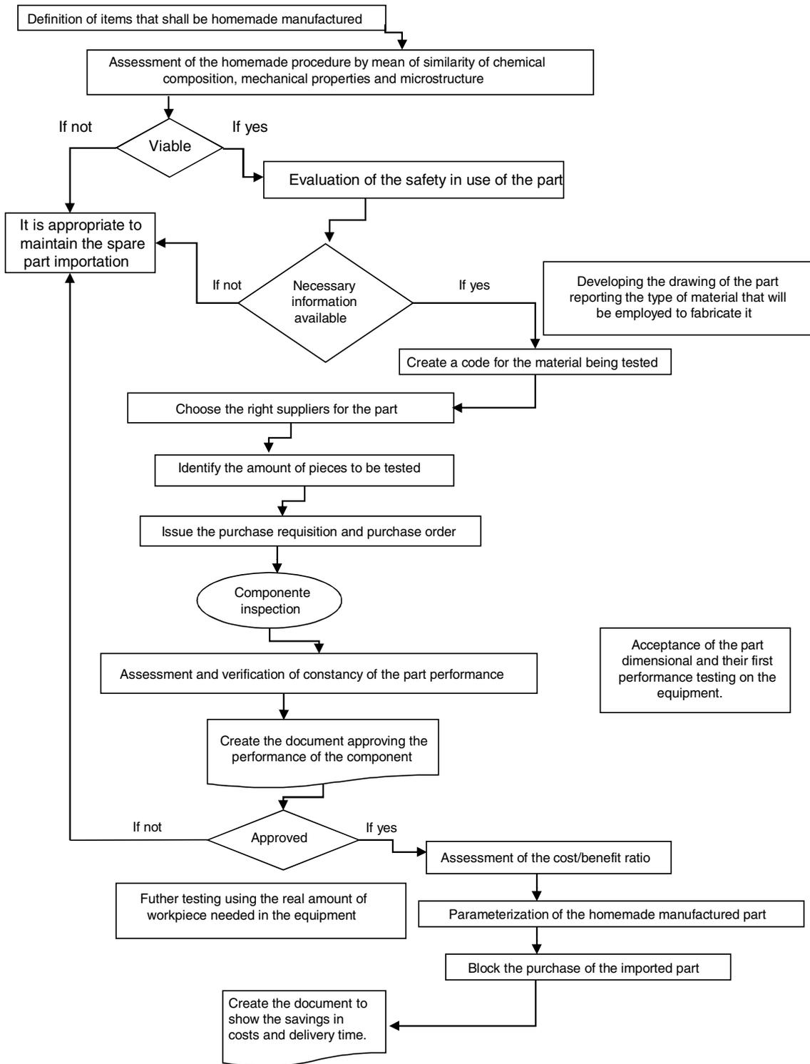
Fig. 2 – The sequence of activities developed during the homemade procedure for manufacturing of the rod part.
